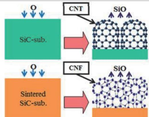
Fig. 1 CNT and CNF (Carbon Nano Fiber with nanoporous) by SiC surface decomposition
