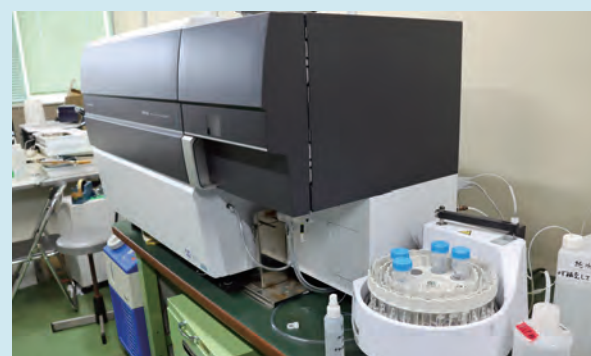
▲ICP発光分光分析装置 Simultaneous ICP Atomic Emission Spectrometer
