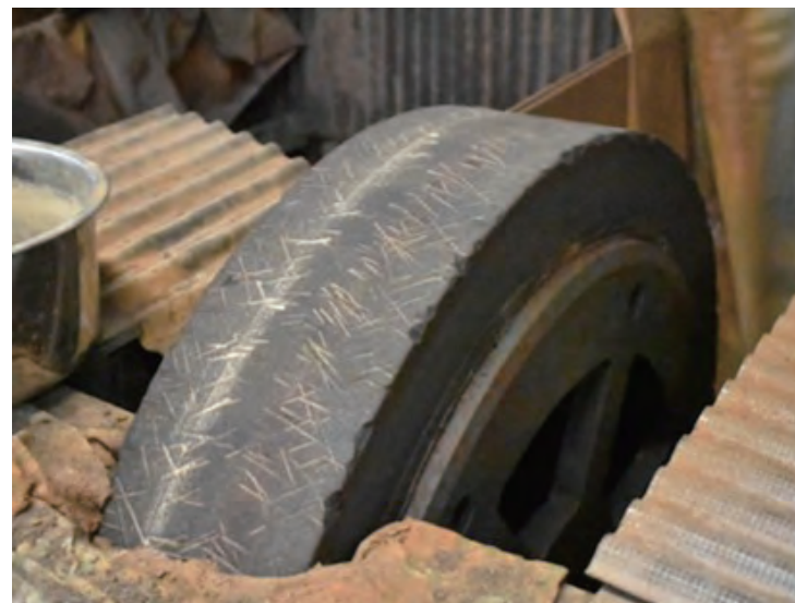
Sharpen it with ENTO, a big rotating whetstone, to make the blade thin.
