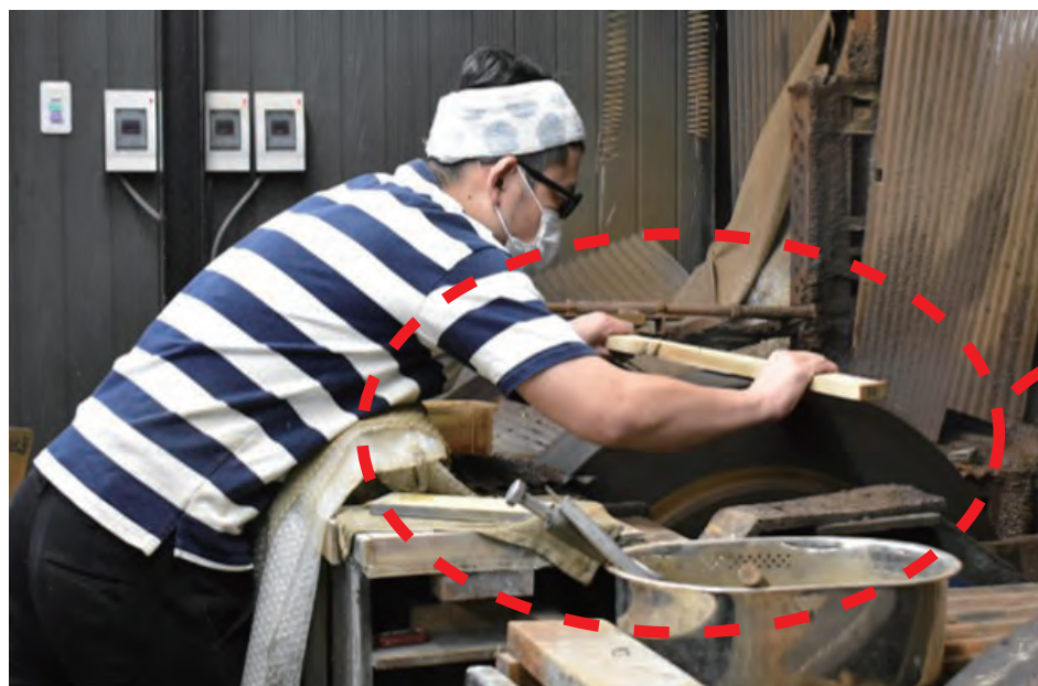
Sharpen it with ENTO, a big rotating whetstone, to make the blade thin.
