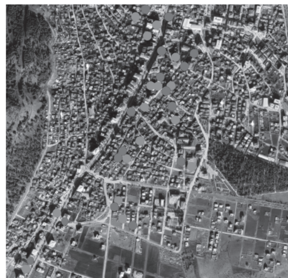
Figure 3. Location of 32 buildings at Islayihed district (Gaziantep province) after the 2023 Türkiye-Syria Earthquake used in the seismic safety exercise at the workshop. The dark grey color represents 16 collapsed housing. The light grey color indicates 16 safe housing. Source: Adapted from Google Maps.
