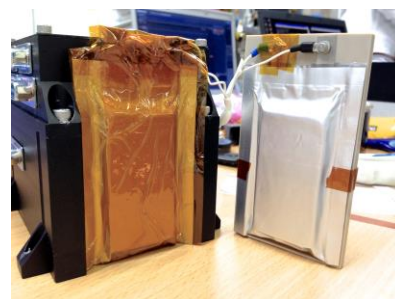
Ionic liquid lithium secondary battery developed by Professor Ishikawa, et al. of Kansai University (top) and the ionic liquid lithium secondary battery that was mounted on the technological demonstration module of HODOYOSHI-3. It is capable of operating under extremely high vacuum with only a simple laminate armor (bottom).
